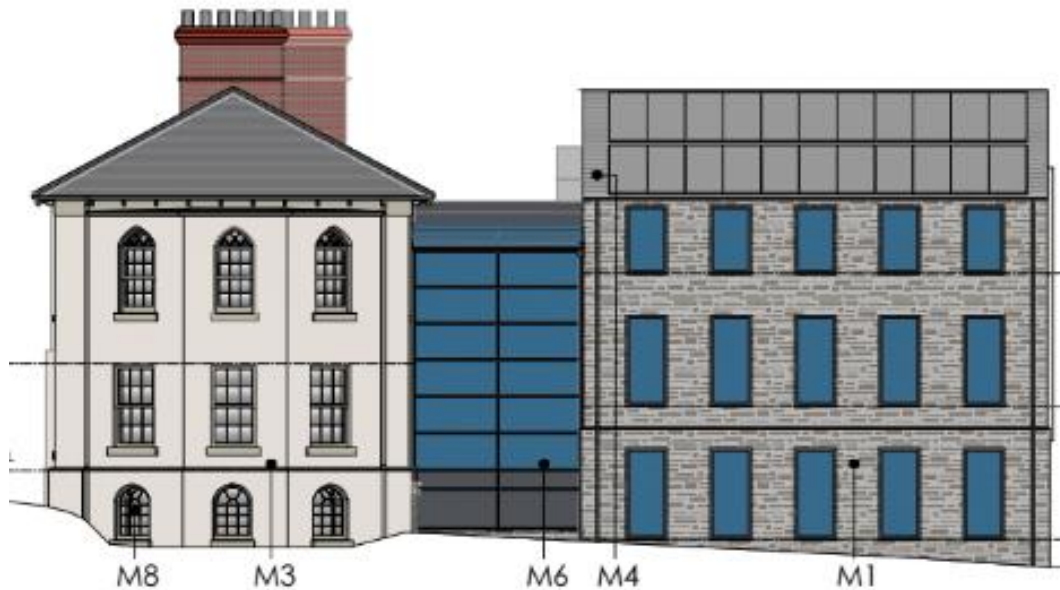
Figure 53 Proposed south elevation showing remodelled Priory House, modern addition removed to the east and new office block added © Gaunt Francis Architects
