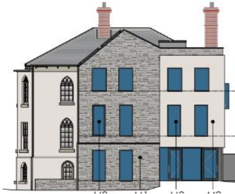
Figure 56 Proposed east elevation showing remodelled Nash building, modern addition removed to the east and new office block added and set back © Gaunt Francis Architects
