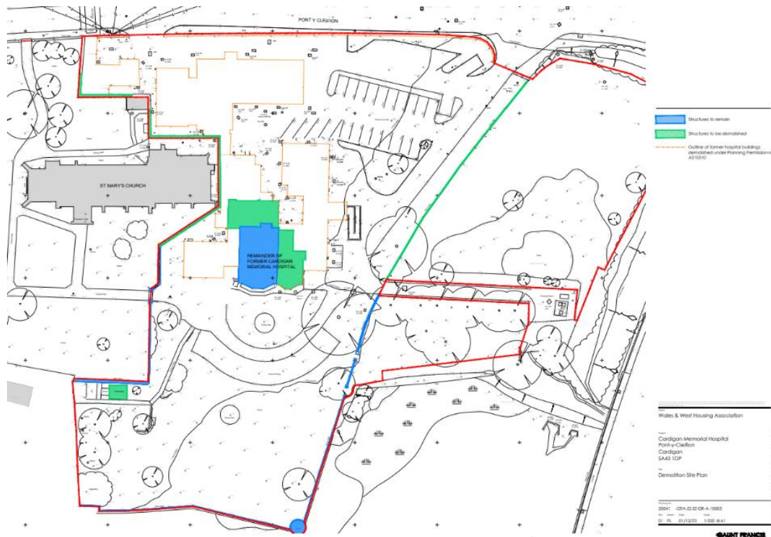
Figure 52 Demolition Plan showing structures to remain (blue) and those to be demolished (green) © Gaunt Francis Architects
