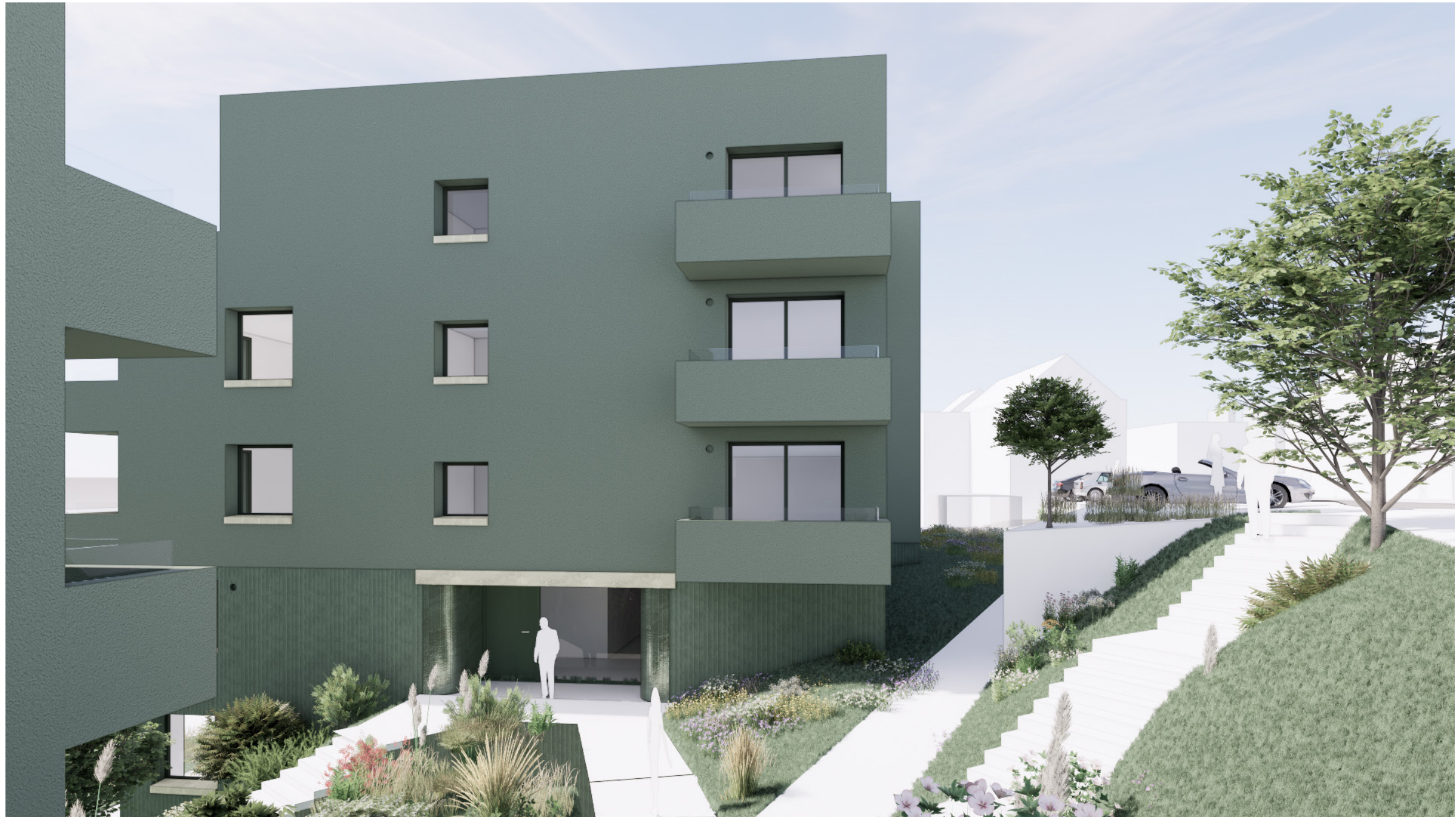
Sketch view showing the garden and entrances to the homes. Ramped and stepped routes are provided to ensure the homes are accessible for all.
