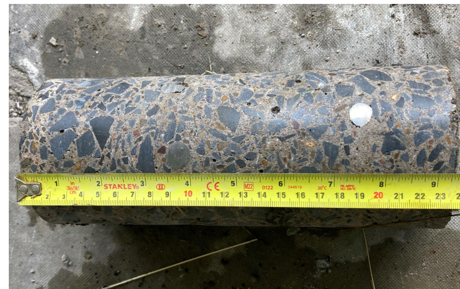
Concrete core log
