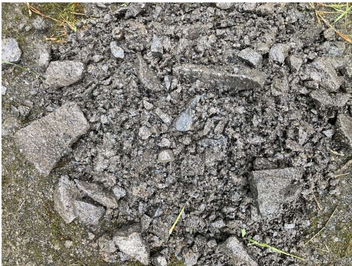
Figure 6-D: Made Ground encountered beneath surfacing in BH04
