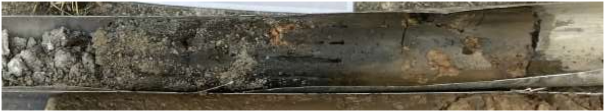
Figure 6-C: Made Ground excavated from BH02
