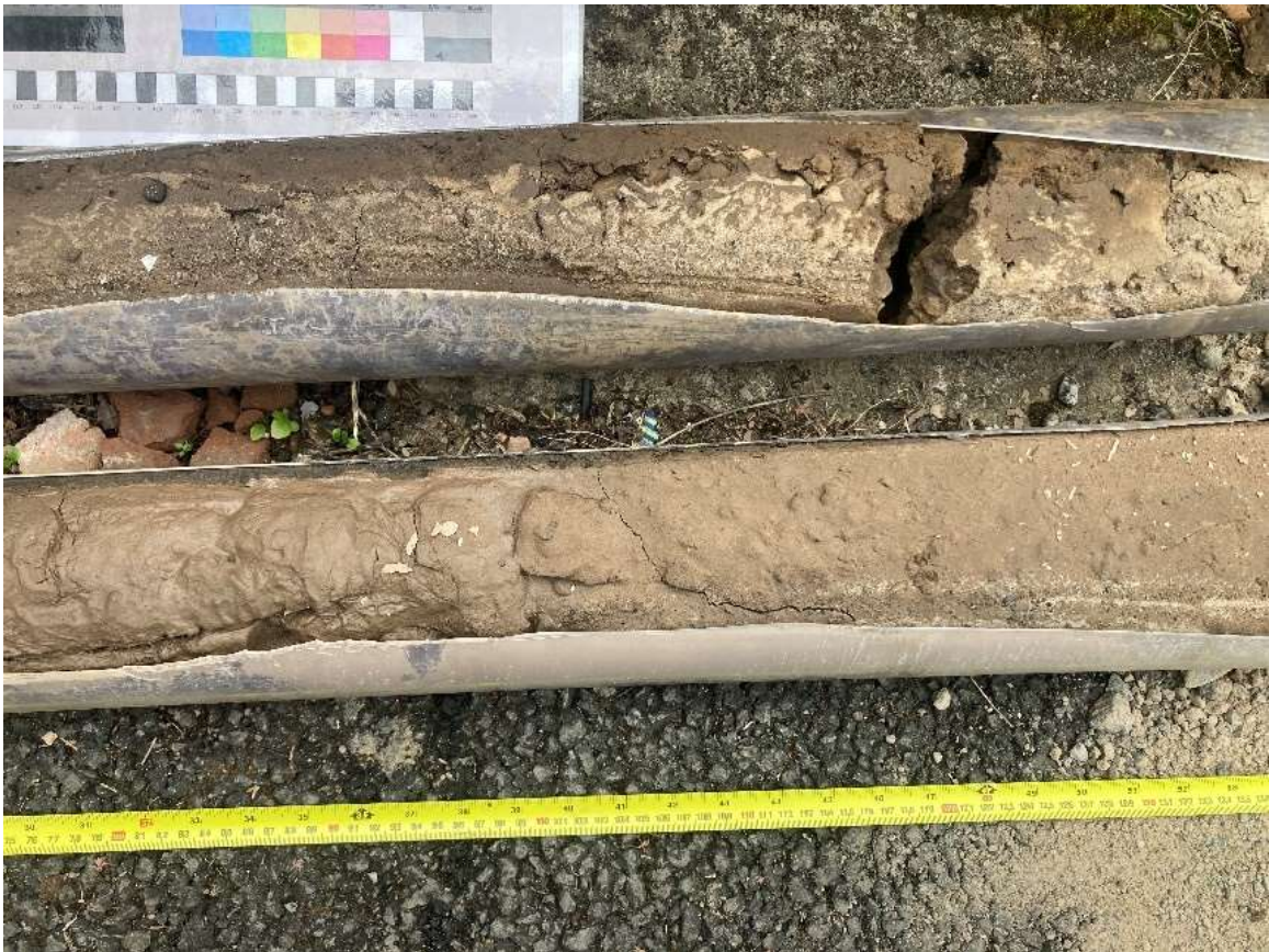
Figure 6-E: Devensian Till excavated from BH01
