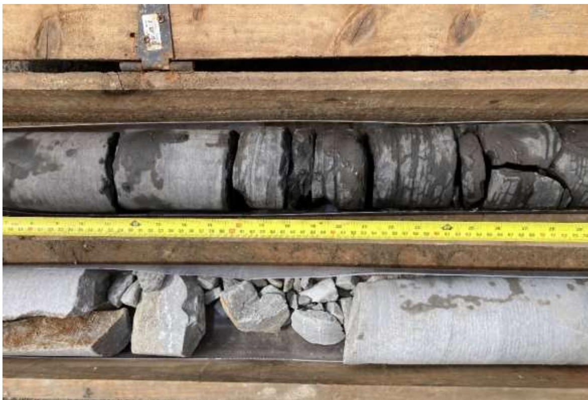
Figure 6-F: Bishopstone Mudstone Formation encountered between 10.5m and 13.5 within BH01
