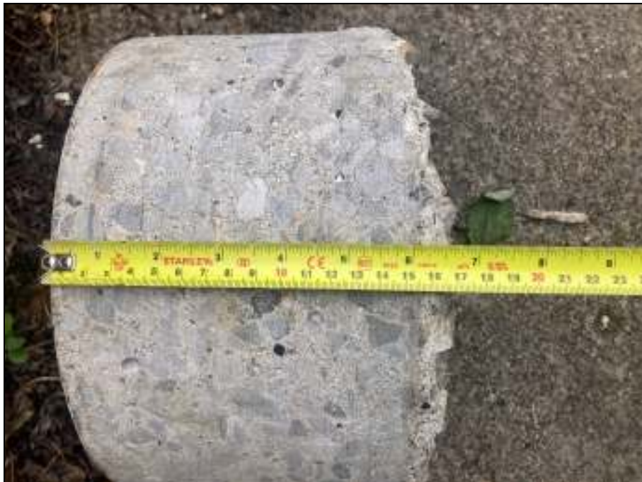
P2: Photograph showing Concrete encountered in BH01
