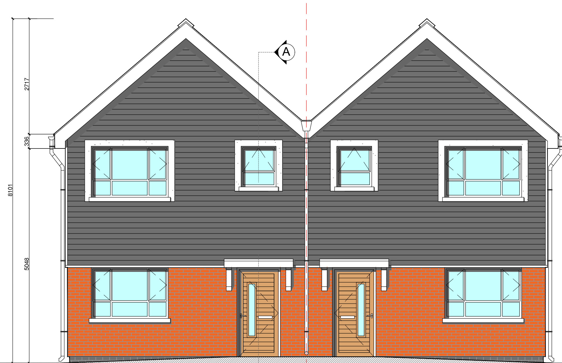
EDRYCHIAD BLAEN FRONT ELEVATION - 1:50
